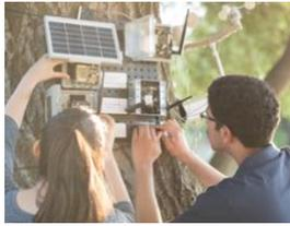
In California, two high school students invented a device to predict the probability of a forest fire occurring (Shah, 2018). The device is placed in the forest and takes real-time photographs and measurements of humidity, temperature, carbon monoxide/dioxide, and wind. This data is then used with a deep learning neural network to predict the probability of a fire.
